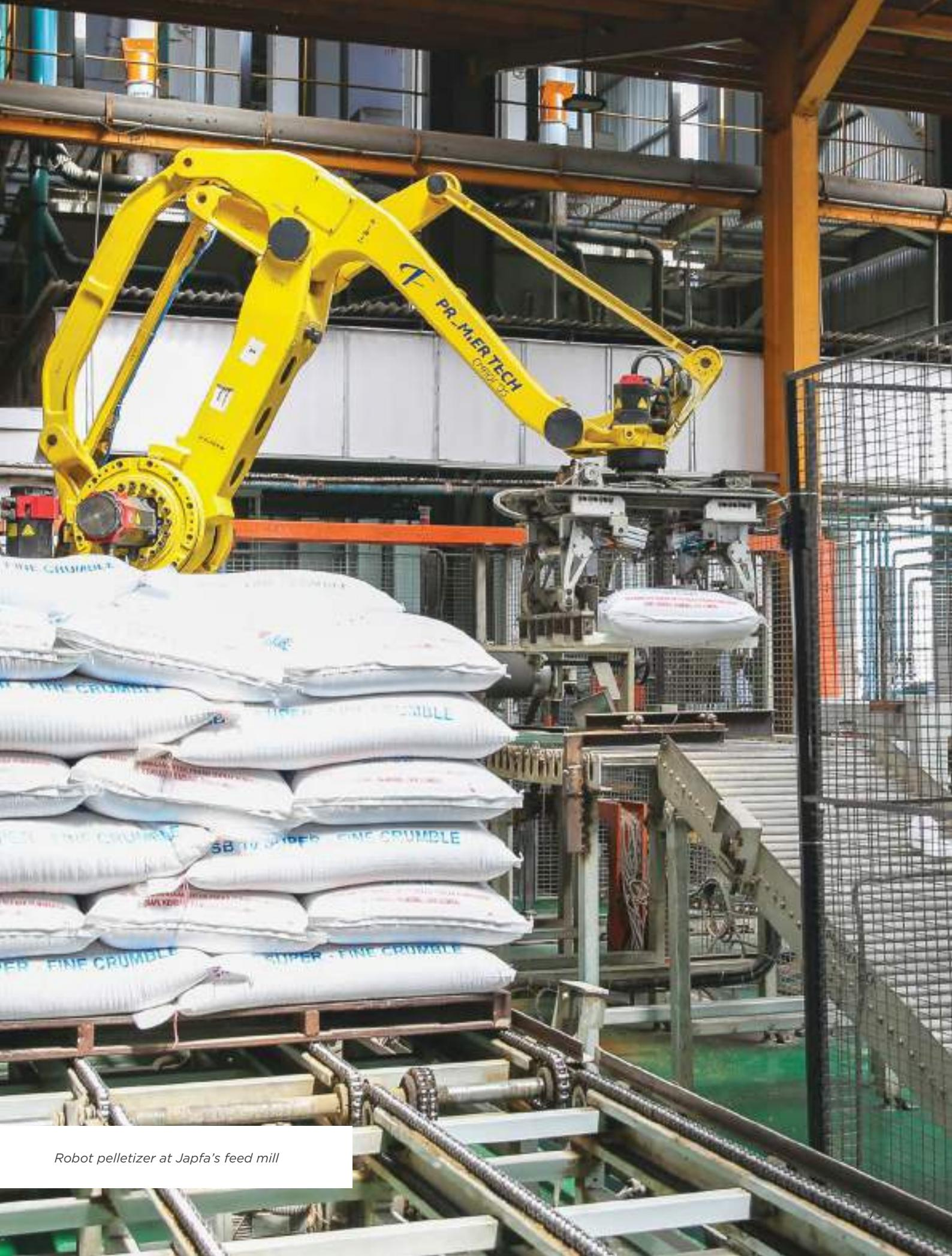
Robot pelletizer at Japfa's feed mill
